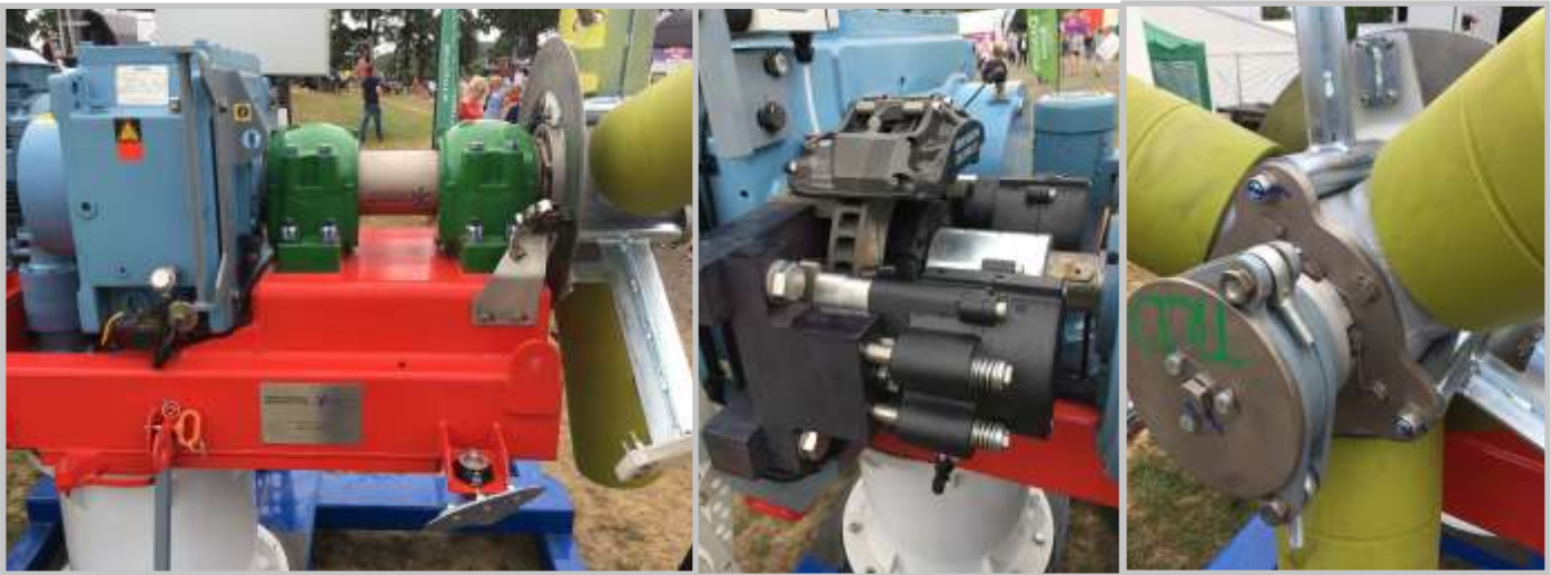
E-Series upgrades, left to right: New bedplate and shaft, upgraded braking system, new hub fastening design
