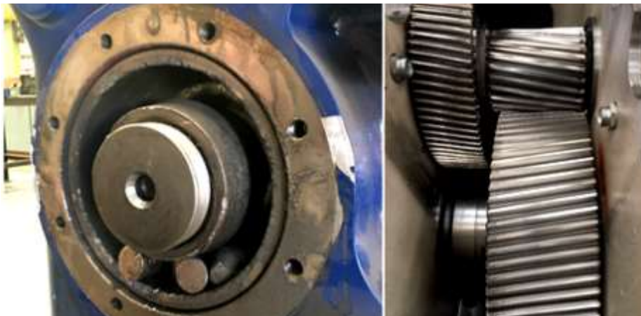
Damaged bearing and gearing in an X35 gearbox
