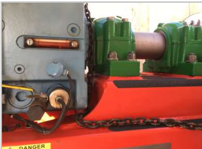
New shaft and bed plate inside the refurbished nacelle
